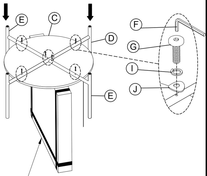
**Attention:** When attaching all legs to the shelf, use the carton from the packaging or a work surface to create a gap between the floor and the legs. This will allow the legs to easily be assembled and properly tightened.
